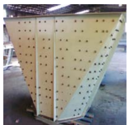
Chute with liners
